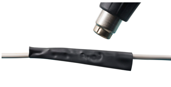
4- Chauffez la gaine thermorétractable
